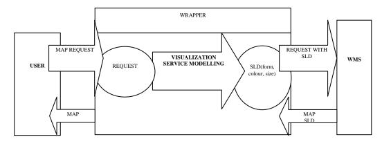
**Relationship between Geosismo and Geoserver.** Geosismo is interrelated with Geoserver so as to extract information about the features corresponding to the parameters introduced by the final user:
